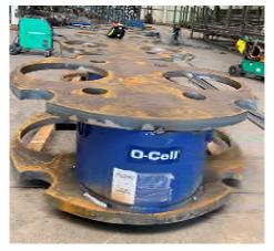
Full scale static load testing using Osterberg-cells was planned as the method is specifically appropriate for the test loads required and on piles of this size and bearing capacity. The results allow confirmation and potentially optimisation of their foundation design without the need for costly and time-consuming installation of the reaction piles used in conventional load testing.
